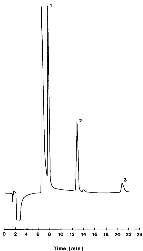
Fig. 2. Indirect conductometric detection of ingredients in cough-cold syrup No. 3. Peaks: 1 = phenylephrine hydrochloride ( 0.4 \mu\text{g} ); 2 = dextromethorphan hydrobromide ( 0.4 \mu\text{g} ) and 3 = chlorpheniramine maleate ( 0.08 \mu\text{g} ). Excipient peak at about 7 min.
